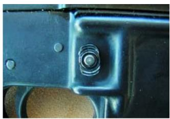
The AR's magazine release is a button located on the right side of the receiver. For speed loads, the author feels this is a better system.
