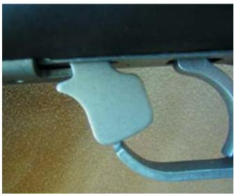
The Mini-14 safety is similar to the Garand, i.e. inside the trigger guard.
