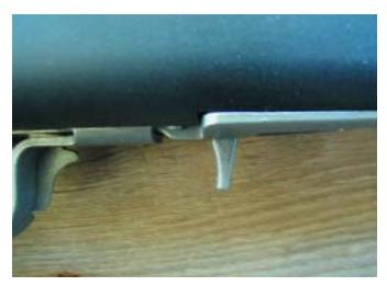
The magazine release for the Mini-14 is the lever-type, located behind the magazine.
