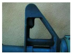
The AR's front sight is enclosed and protected by "wings."
