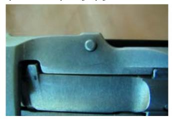
The Mini's bolt hold-open device is a button located on the top left of the receiver.
