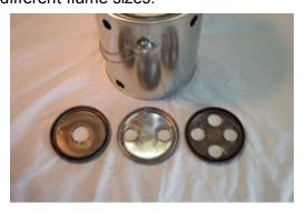
**STEP 8. Extinguish the stove.** Remove the cooking pot from the stove. Using a pair of long nose pliers remove a few support grills. Using the pliers again grab the lip of the quart can lid and carefully place it over the burner, smothering the flame. Wait a while allowing the stove to cool down before touching the stove.
