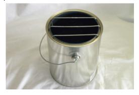
**STEP 3. Make the air holes.** Using your Uni-bit, drill 4 air holes (about 1/2" diameter) around the top rim of the gallon paint can. Then drill 2 to 4 air holes around the bottom rim of the can. Note: you can also create the air holes using a church key can opener.
