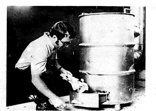
Lighted paper is inserted into the drawer to ignite the sawdust stove.
