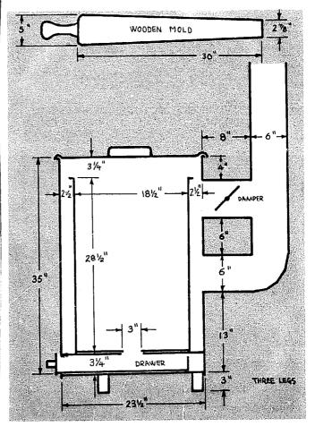
Figure 2.—Design of the experimental doubledrum stove.
