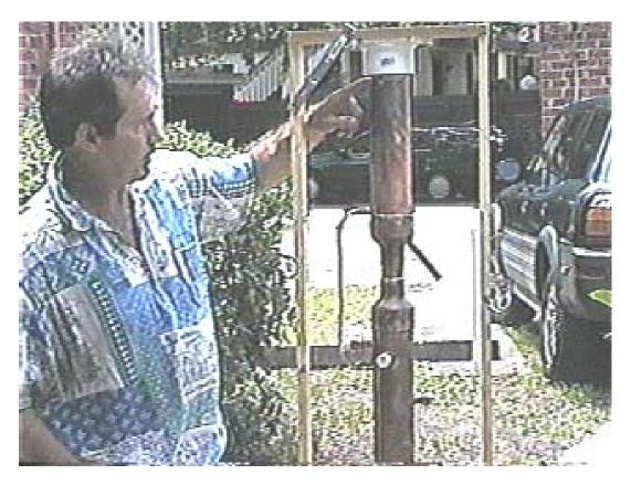
Here, I used a PVC toilet floor flange to secure the top and bottom ends of the still to the frame. The white thing in front, middle, is a white plastic plug I installed temporarily to close the hole where the temperature gauge will be installed (and keep the marbles inside).
