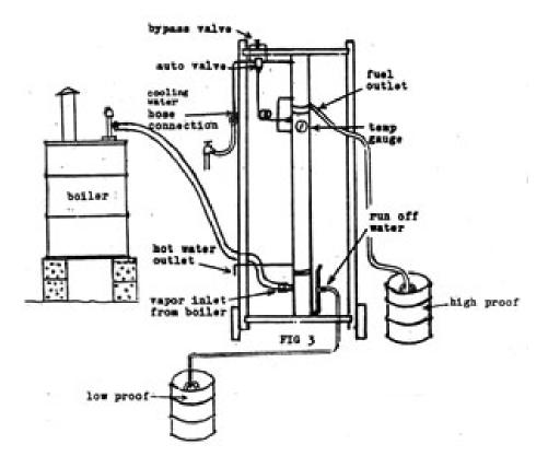
The boiler should present the largest liquid surface area possible. Vapor comes out of the liquid only at the surface, so the more surface area, the greater the opportunity for the vapor to leave.
