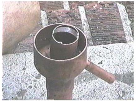
On the top of this smaller 1-1/2 inch pipe which you see in this photo is where you will attach a couple curved strips of copper to keep the marbles from the bottom section from rolling into the top section if you lay the still down into a horizontal position for carrying it. The smaller  $\frac{1}{2}$  inch pipe on the lower right of this photo is the high-proof fuel outlet.
