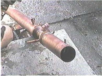
Top of condenser section with coil inserted.
