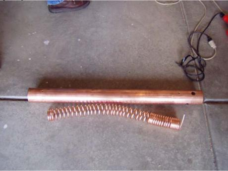
**20. Inserting the cooling tubing**. Now you need to unwind just a little of each end of this coil, and then pull on the very last coil so that you are pulling the straight end of the
