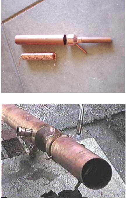
This is the condenser section being soldered into place, after gently tapping it inside the 3-inch midsection joint. Read on further, as it doesn't get attached yet.
