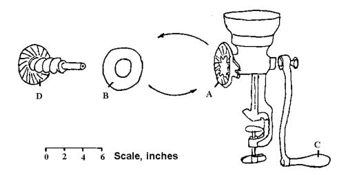
Hand operated rice huller: A) stationary disk, B) rubber disk, C) handle and D) rotating disk with auger. Remove stationary disk and replace with rubber-faced disk.
