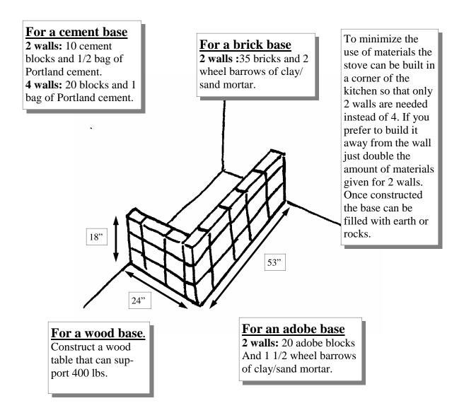
**NOTE**: Adobe blocks are the most environmentally friendly option for building the base and the body of the stove because adobe blocks are not fired like clay bricks. The plans use bricks only because, in the USA, and in many parts of Latin America, fired bricks are easier to obtain than adobe blocks.
