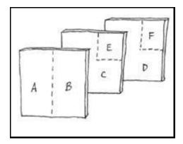
Take three baldosas (1" by 12" by 12"). Cut all 3 tiles to 1" X 10" X 10". Cut the AB tile in half. This will leave you with two 5" by 10" pieces. Then take the second tile (CE) and remove a 5" by 5" square (E) and then take the third tile (DF) and remove a 5" by 5" square (F).
