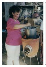
The single-pot Rocket stove is less expensive and more efficient (25- 30%) than the Justa Stove. It is ideal for cooking outside or in areas where a chimney is not needed or available.
