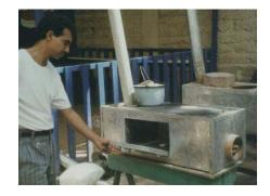
This metal Justa with oven is being constructed by Ahdesa in Honduras and by Prolena in Nicaragua. The metal Justa is approx. 30% more expensive but it allows for mass production and ease of transport.
