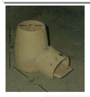
The combustion chamber can be made from refractory cement, refractory ceramic, 1/8th" steel, or cast iron. We are also experimenting with a ceramic tile (see page 7) from Guatemala and our own refractory mix.
