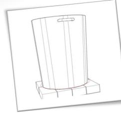
**Step 1**: Arrange your fire bricks into a square, then place the dustbin on top and use it to trace the outline of the base onto the bricks with chalk. You will need to use an angle grinder, with a masonry cutting disk fitted, to cut them to shape so they fit inside the dustbin.
