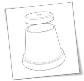
**Step 3**: Turn your plant pot bottom side up, and measure about 3cm. Use your angle grinder, with a masonry cutting disk fitted, to cut away the top, save it as you will need this later to cover your oven.
