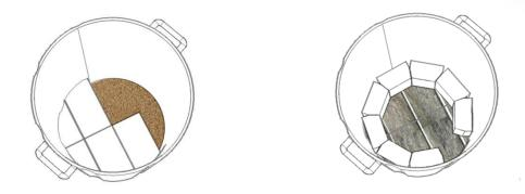
**Step 5**: Now that you know the depth required, place the appropriate amount of sand into the bottom of the dustbin and arrange your fire bricks inside onto the layer of sand. Arrange the remaining bricks around the edge of the dustbin, leaving a gap approximately the size of one brick. This forms an air vent and allows removal of ashes.
