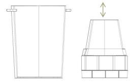
**Step 4**: Stand your plant pot onto the firebricks and place it next to the bin. Ideally the top of your plant pot wants to be level with the top of the Dustbin. Compensate for any height difference using sand once it is inside the dustbin.
