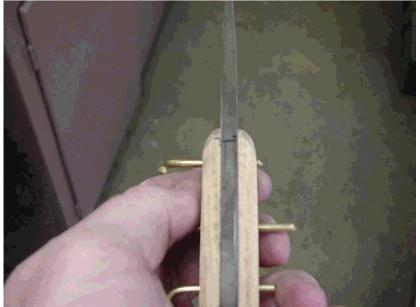
At this point if you have nice flat slabs and no gaps between the slab and the metal you are ready to cut some pin material just enough to stick out past the slab on each side. Degrease the blade good where you are going to place the slabs. Dish soap and hot water with an old toothbrush then rinse real good and wipe dry. Hit it with the hair dryer for a few minutes if you want to make sure it is completely dry.
