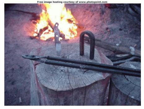
Put that blade in the hot coals. It will take about 10 to 15 minute depending on how many and how hot the coals are. It is your first so pull it out and look at it for a couple of seconds every 2 or three minutes and check it with the magnet on the cutting edge from tip to plunge. If the magnet has a pull on it it is not ready to quench put it back and let it get cherry red. Try not to heat it any longer than is needed by checking every minute or two when you think you are close.
