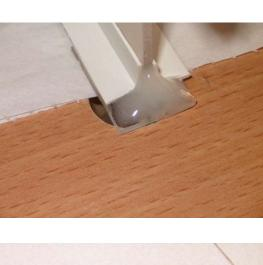
Le the glue dry, then fill the surrounding sace with blu-tack to stop light leaking.
