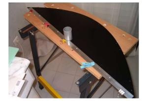
Adjacent angles are fixed by a bolt at the corner of the cover. This picture also shows the gap between the edge of the plate and the vertical side of the end angle.
