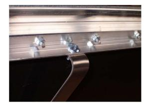
Global view of the back after the edge redressing mechanism being installed.
