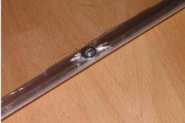
To protect the outer surface of the cover against scratches, the easiest method is to put a thin plastic film on it. The plastic food wrap is good for this, but a thicker one would be better. Care must be taken not to leave air bubbles between the film and the plate. There will be no light loss if there is no air bubbles.
