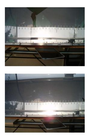
By the way, the above two pictures show an image of the receiver which is still quite straight and regular near the edge of the collector. This image is an important indicator of the optical quality of the collector, and at the same time a difficult one. The reader can compare this to the large number of published pictures of other parabolic troughs, in order to appreciate the quality of this realisation: the others usually give far worse images.
