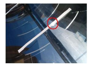
Or for checking leaking coming from edges of the mirror, a flat plate can be used. Here the lower portion of the plate is illumated by some slight leaking from the upper edge of the collector, due to the double reflection phenomenon (see below).
