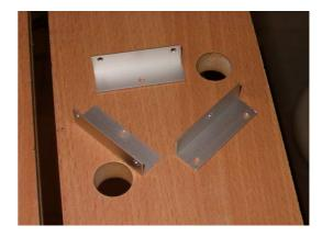
Fasten five above pieces on each end of the back, each fixed by one 3mm bolt, with the head of the bolt on the reflective surface.
