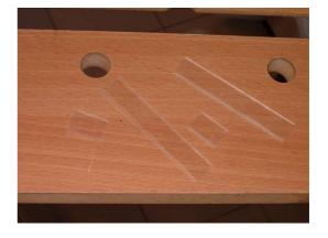
Thoroughly scratch the surfaces of the two longer bars with coarse sandpaper, to create a scattering effect.
