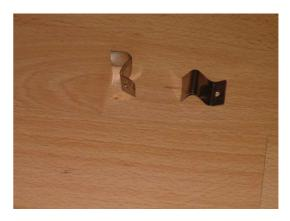
Use a nut to fix the holder on the side angle of the cover, to prevent the detachment of the back. Note that the holder should not put pressure on the side angle of the back, in order not to deform the latter. So a small moving space should be left between the holder and the side angle of the back.
