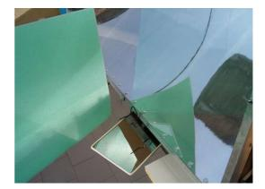
In any case, a leaking of sunbeam means defocussing and loss of collector efficiency. Therefore sunbeam leaking must be kept to as little as possible, by correcting the causes. Each type of leaking has its particularities and causes.
