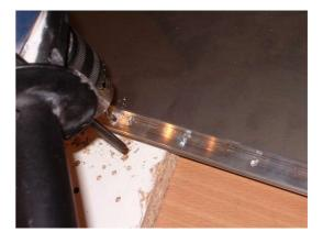
Fasten the side angles on the back using 3mm bolts and washers as shown, one at each side. Check that the tails of the bolts do not exceed the straight line joining the two outer edges of the angle. If they exceed, the exceeding part must be cut off.
