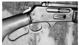
AKey Marlin features: side ejection port, traditional loading gate, crossbolt (push button) safety, and extended hammer for easier cocking.
