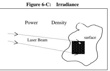
second). A typical laser rangefinder emits 60 millijoules ( $60 \times 10^{-3}$  joules) of energy in a 20 nanosecond ( $20 \times 10^{-9}$  seconds) pulse. The irradiance is expressed in power per unit area, watts/cm<sup>2</sup> (see Figure 6-C). The laser irradiance is one of the critical parameters in determining the effects a laser will have on an object such as an eye.
