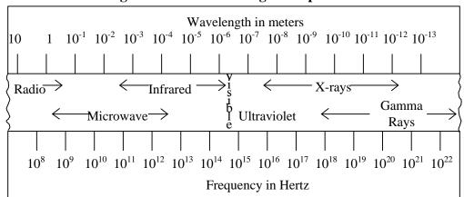
Figure 6-B: Electromagnetic Spectrum
