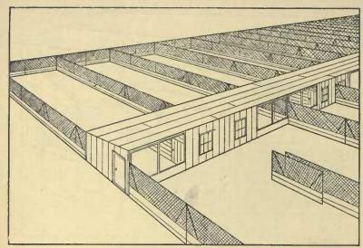
Fig. 11 - Continuous scratching-shed poultry house, with double yards.
