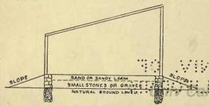
Fig. 1 - A plan to secure dryness.
