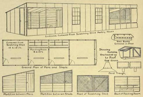
Fig. 14 - Continuous curtained-front, scratching-shed poultry house.
