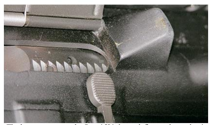
The brassy smear on the Stag 15L's brass deflector shows that it works as designed.
