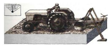
The mole drainer A torpedo-shaped steel object at the bottom of a narrow blade is dragged through the soil. The narrow slot made by the blade fills in but the drain remains. The drain lasts much longer in clay than in soft sandy soil.
