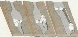
**Positioning and** types of dam In order to build up a head of water and control its flow, it is often necessary to build a dam or a weir (above) across the main stream, usually at a narrow point or where there are rapids. A head race or leat, dug along a contour above the stream, will create enough head for a water wheel or turbine to function. A dam can be a pile of rocks in a stream, although wooden dams (below right) or combined wood and earthfill ones (right) are effective.
