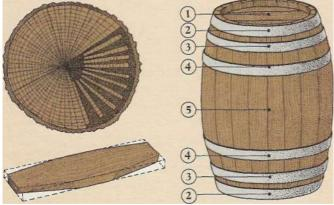
The parts of a barrel
