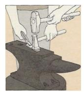
chopping, because its surface is softer and will not suffer damage. The "beak", the long pointed bit, is for wotking anything that needs a curved edge. To flatten metal, or remove marks made by a hammer or other tool, you should hold hot metal on the face of your anvil with tongs, hold a flatter over it and whack it with a sledgehammer until you achieve the desired effect.
