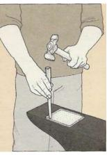
The hammer and pritehell To make holes in any metal, and particularly in horseshoes, you should use a pritehell, which is a square-handled punch. Again use this on your anvil's face and hit it with a heavy blacksmith's Warrington pattern hammer (above), or with a ball pane hammer. If you need to make a large hole, do it over the round hole in the "tail wedge" of your anvil to avoid damaging the table underneath.
