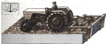
The chisel plough Tv; chisel plough, or subsoiler, cuts - s€-.~s of deep, evenly spaced =i < in the soil. This works very •-•£- u ith heavy clay, where the -»~: u 5 last and ensure free
