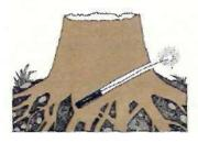
**Blowing up a stump** Put your charge in a hole deep under the stump and retreat.
