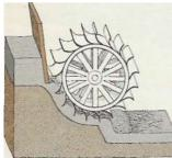
**Breast wheel (undershot)** An undershot wheel with straight blades is up to 30% efficient; fitting curved blades increases this to 60%. A breast wheel makes twice the power from the same source.
