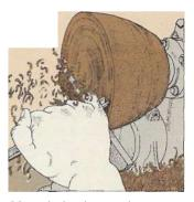
Move the handrest so that you can work on the inside. The unbreakable rule for hollowing wood on a lathe is: begin at the outside and work towards the centre. Start with a gouge, then scrape with roundended scrapers only, and finally sandpaper it smooth. Remove the chuck from the lathe, unscrew it and fill the holes with plastic wood. Polish the whole thing with beeswax and glue felt on the bottom.
