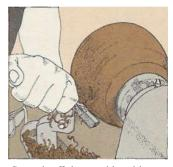
Smooth off the outside with your scrapers. Then, keeping the bowl on the lathe, rub with sandpaper, which will give the wood a gloriously smooth finish.
