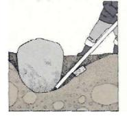
Use a rock or a chunk of wood as a fulcrum. Work a lever down beside the boulder.
