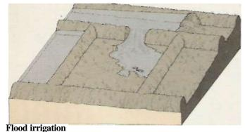
Sloping beds, previously levelled, with a water channel at their head, are separated by little earth bunds. You make a dam across the channel at the first bed, break the bund separating channel from bed, close the gap once the bed is flooded, destroy the dam and repeat the process.
