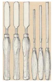
must replace the stock with a rod fixed to a chuck to which the bowl can be attached. For the heavywork of removing unwanted wood you need three gouges of differing thicknesses (above right), and for the more delicate shaping and smoothing you need scrapers (above left). Never press hard with any tool, particularly a gouge. If they stick you are in trouble. Keep your tools sharp. Factory-built lathes often have a revolving sharpener built on. Otherwise use an oilstone.
