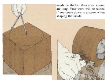
Take a block of wood, mark the centre with a cross and draw a circle with a compass slightly larger, say + inch (6 mm), than the intended diameter of your bowl.
