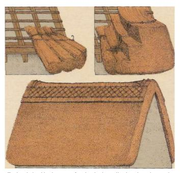
To thatch the ridge lay arowof yealms horizontally along it, and cover them with more yealms folded over the ridge and secured on both sides with sways, brottches and hooks. You can use hazel sways to decorate the roof.
