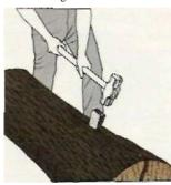
made until the log splits right down its length. Never use an axe as a wedge. The handle will break.
