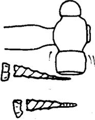
Bend each end in the direction of the edge (not the face) of the flat side.
