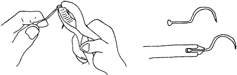
**Tweezers:** Draw the shape on a piece of tin and then cut it out with strong scissors. Use a file or a smooth stone to make the edges smooth. Bend in half to make the tweezers.
